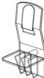
Locks base shelves in place and prevents shelves from sliding. Designed to allow easy shelf removal. Molded from clear high-strength polycarbonate. Standard feature on all base and tall cabinets.
